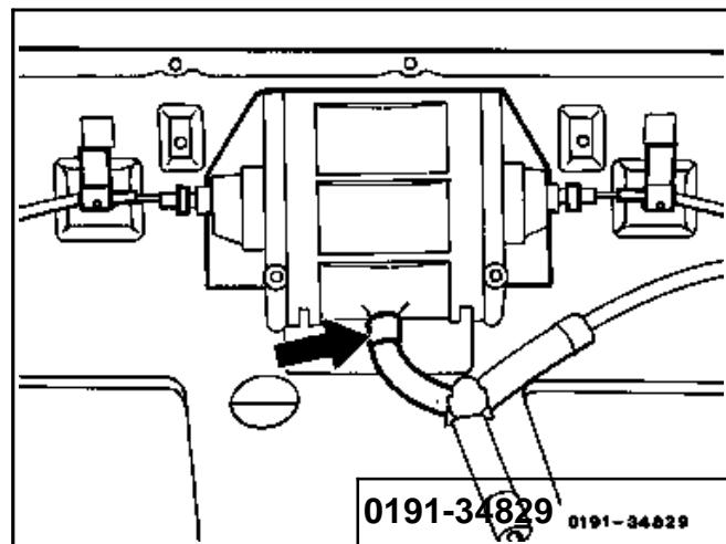
4 Disengage both cable controls on vacuum element, take off lock for this purpose and also remove clamp for attachment to cushion frame from clips.
