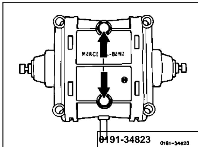
**Note:** When engaging both cable controls, make sure that the cable control envelopes are uniformly projecting for approx. 7 mm on clamps.
