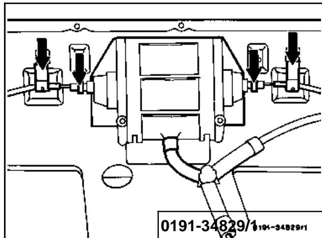
5 Loosen 8 mm screws (2 each) on vacuum element, push slightly toward the rear and remove from cushion frame.
