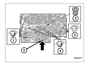
7. Install the strainer (1) in the inlet to torque converter lock-up control solenoid valve.
