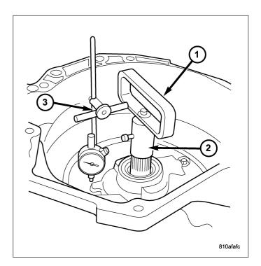
e. Move input shaft in and out and record reading. End play should be 0.3-0.5 mm (0.012-0.020 in.). Adjust as necessary.
