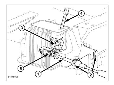
6. From under the hood, route the gearshift cable (1) forward of the air conditioning lines and the heater hoses (2) and toward the transmission (3) manual lever.
