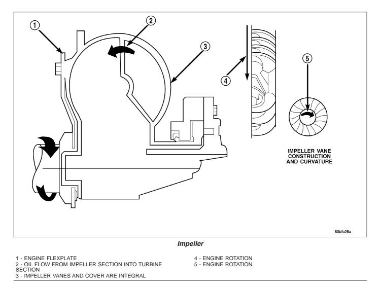
The impeller (3) is an integral part of the converter housing. The impeller consists of curved blades placed radially along the inside of the housing on the transmission side of the converter. As the converter housing is rotated by the engine, so is the impeller, because they are one and the same and are the driving members of the system.
