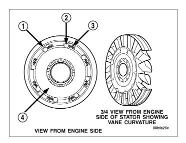
The stator (1) is located between the impeller (2) and turbine (4) within the torque converter case. The stator contains a freewheeling clutch, which allows the stator to rotate only in a clockwise direction. When the stator is locked against the freewheeling clutch, the torque multiplication feature of the torque converter is operational.
