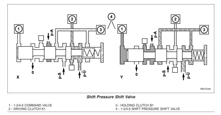
Each shift group possesses one shift pressure shift valve (4). The 1-2 / 4-5 and 2-3 shift pressure shift valves are installed in the shift valve housing; the 3-4 shift pressure shift valve is installed in the valve housing. It assigns the shift pressure (p-S) to the activating actuator and the overlap pressure (p-Ü) regulated by the overlap regulating valve to the deactivating actuator.
