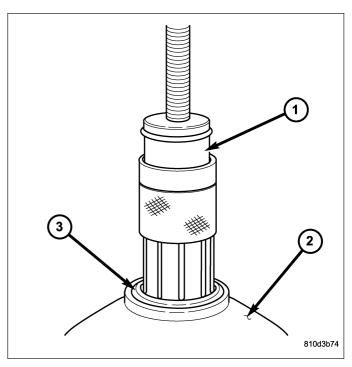
9. Slide the collar (3) on the Bearing Remover 9082(1) downward over the fingers (3) of the tool.
