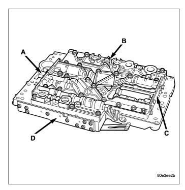
Note: Pay great attention to cleanliness for all work on the shift plate. Fluffy cloths must not be used. Leather cloths are particularly good. After dismantling, all parts must be washed and blown out with compressed-air, noting that parts may be blown away.
