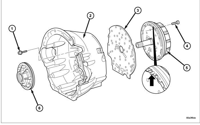
Install Holding Clutch B1 and Oil Pump
