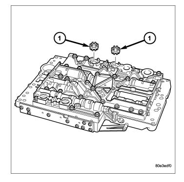
14. Remove the strainer (1) in the inlet to torque converter lock-up control solenoid valve.
