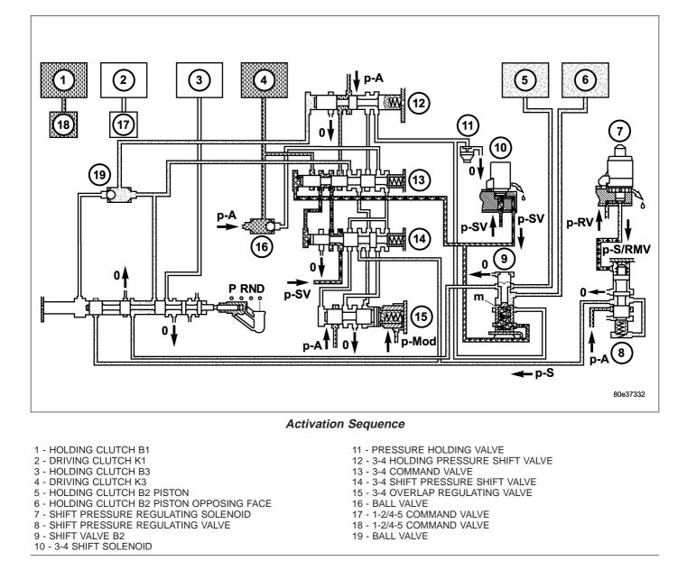
The selector valve opens the shift pressure (p-S) feed connection from the ball valve (19) with the shift valve B2 (9). With the shift valve B2 (9) in the upper position, shift pressure (p-S) travels behind the piston B2 (5) and simultaneously to the opposing face of the piston B2 (6). The multiple-disc holding clutch B2 begins to close.
