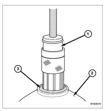
14. Slide the collar (3) on the Bearing Remover 9082 (1) downward over the fingers (4) of the tool.
