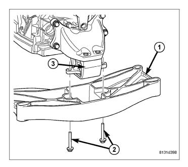
Install the transmission (3) to engine oil pan (2) bolts (1). Tighten to 39 N·m (29 ft.lbs.).
