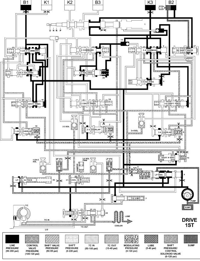
HYDRAULIC FLOW IN DRIVE - FIRST GEAR
