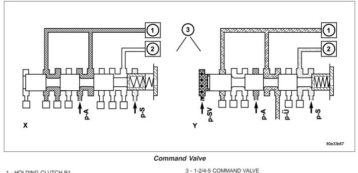
1 - HOLDING CLUTCH B1 2 - DRIVING CLUTCH K1
