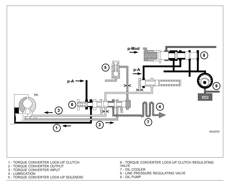
The torque converter lock-up clutch regulating valve (6) is located in the valve housing of the electrohydraulic control module. The valve is responsible for the hydraulic control of the torque converter lockup clutch and distribution of the lubricating oil.
