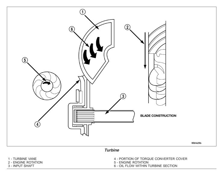
The turbine (1) is the output, or driven, member of the converter. The turbine is mounted within the housing opposite the impeller, but is not attached to the housing. The input shaft is inserted through the center of the impeller and splined into the turbine. The design of the turbine is similar to the impeller, except the blades of the turbine are curved in the opposite direction.
