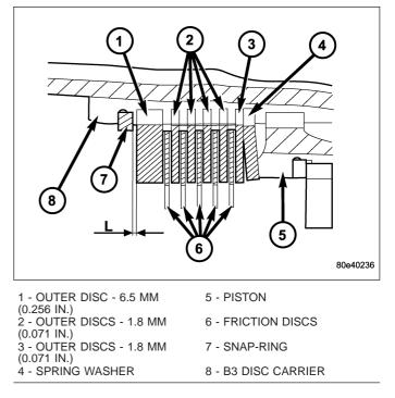
Applying excessive force to the clutch will give an incorrect reading and lead to a transmission failure.Using a feeler gauge, determine the play "L" at three points between the snap ring (7) and outer multiple-disc (1). B3 clutch clearance should be 1.0-1.4 mm (0.039-0.055 in.). Adjust the clearance as necessary.
