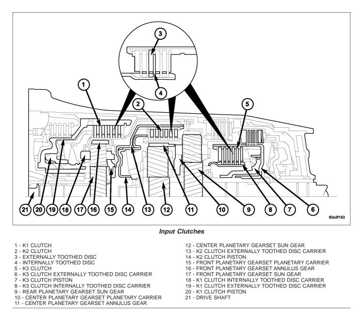
The input clutches produce a non-positive locking connection between two elements of a planetary gear set or between one element from each of two planetary gear sets in order to transmit the drive torque.
