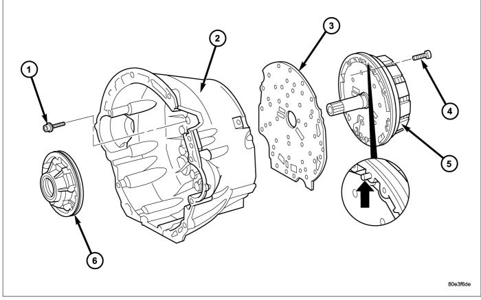
Remove Holding Clutch B1 and Oil Pump
