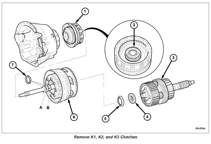
1 - DRIVING CLUTCH K1 2 - SUN GEAR OF FRONT PLANETARY GEAR SET 5 - THRUST WASHER 6 - FRONT PLANETARY GEAR SET, DRIVING CLUTCH K2, AND INPUT SHAFT 7 - SEALING RINGS
