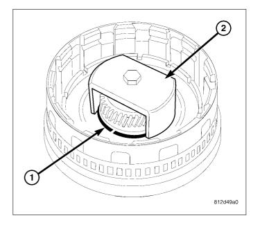
CAUTION: When working with double sided friction discs, an externally lugged steel plate is installed first, followed by a friction disc, and continuing on until all the required discs are installed. When working with single sided friction discs, an externally lugged disc is installed first, followed by an internally lugged disc, and continuing on until all the required discs are installed. All single sided discs are installed with the friction side up.
