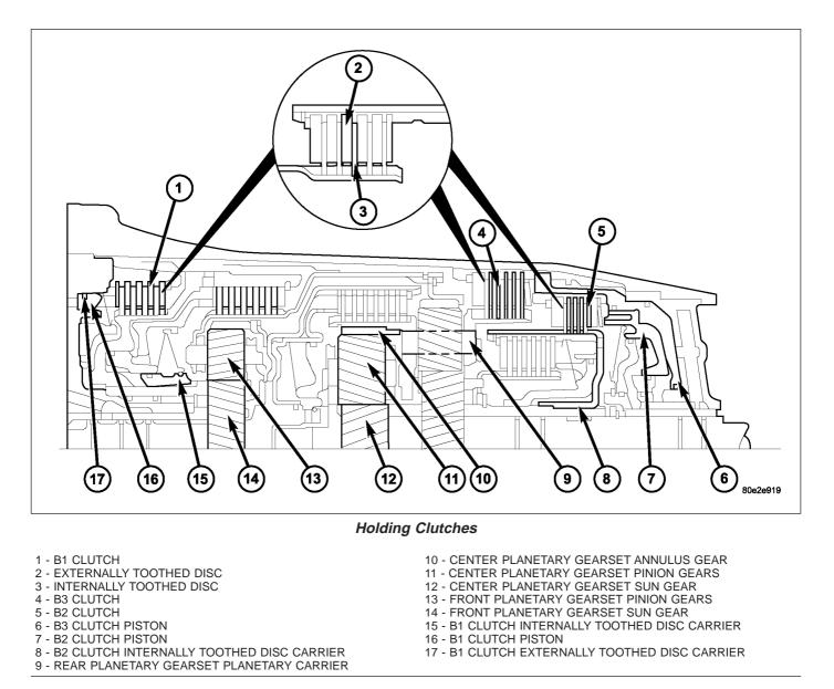
The holding clutches connect the annulus gear, sun gear, or planetary carrier of a planetary gear set against the transmission housing in order to transmit the drive torque.
