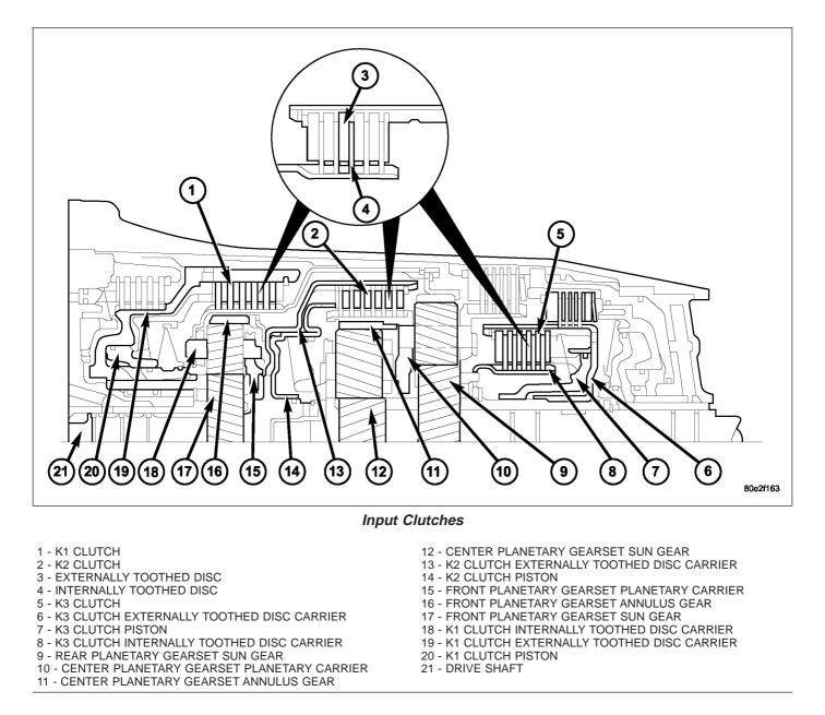
Three multi-plate input clutches (1, 2, 5), the front, middle and rear multi-plate clutches K1 (1), K2 (2), and K3 (5), are located in the planetary gear sets in the transmission housing.
