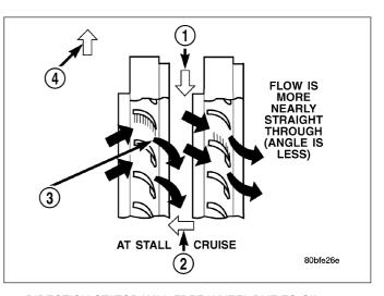
1 - DIRECTION STATOR WILL FREE WHEEL DUE TO OIL PUSHING ON BACKSIDE OF VANES
